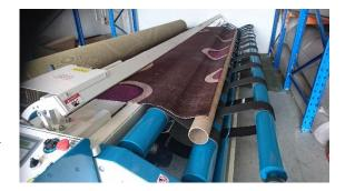
14. Turn the right (cut side) roller switch to Reverse
